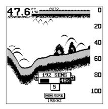
However, you can adjust some features separately when you're using both 50 and 192 kHz. For example, the sensitivity menu shown at right lets you select either the 192 or 50 kHz chart by pressing the appropriate arrow key. To adjust the 192 kHz sensitivity, press the left arrow key. The screen shown below appears.
